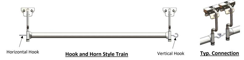
The Railex Hook and Horn linkage is fast and easy to use. The trolleys link together simply by swaying one trolley to the left. This allows for the hook and horn to interlock, but also separate easily.
