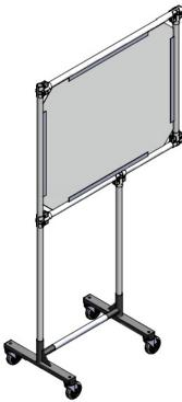
8. 1370-3W6T-C: A cantilever base supported guard that has a shielded area of 3' 6" wide x 3' tall. The base is 2' wide. Ideal for situations where line workers are shoulder-to-shoulder working over a work table or conveyor.
