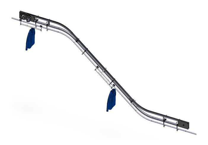
The System 211 is specifically designed for garment manufacturers, garment distribution centers, and uniform rental; to move trolleys between floors, mezzanine and main floors. Suitable for continuous operation. High capacity, 32 ft. /minute up, down, or both. Elevation changes up to 20′ – Incline 30° and 37°. Quiet, lubrication-free operation.
