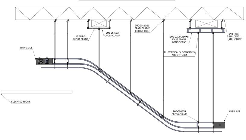
The Railex System 211 is most often suspended from the ceiling. Railex is able to provide a full BOM of all the materials you will need to install your trolley booster rail. Our full line of System 200 Slick Rail fittings and tube is ideal for this application. We encourage our clients to send us sketches or prints of what they want to do in their facility, and we will orient the system into place in your CAD print or we will create one.
