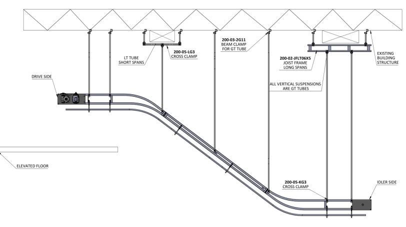
The Railex System 211 is most often suspended from the ceiling. Railex is able to provide a full BOM of all the materials you will need to install your trolley booster rail. Our full line of System 200 Slick Rail fittings and tube is ideal for this application. We encourage our clients to send us sketches or prints of what they want to do in their facility, and we will orient the system into place in your CAD print or we will create one.
